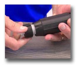
Step 4: Unscrew and remove the check valve nut.
