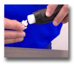
**Step 19:** Now install the new check valve assembly (Part #: PJDI026) into the stem as shown.
