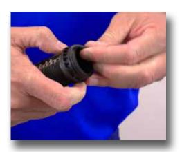
**Step 11:** Then, remove the injection sleeve o-ring (Part #: J024) by pinching and rolling it off of the black sleeve. Install the new o-ring into the groove.
