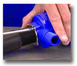
**Step 2:** Unscrew the four screws at the base of the injection stem.
