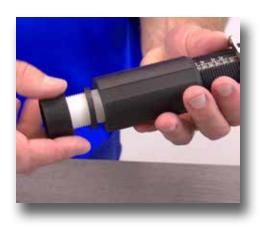
Step 6: Unscrew the lock nut.
