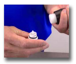
**Step 5:** Pull the check valve assembly straight out of the white stem. Discard the old check valve parts.
