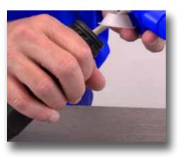
**Step 3:** Pull the stem straight out from the body of the injector. Set the body aside.
