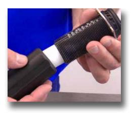
**Step 8:** Unscrew and remove the black adjusting nut. Then, remove the metal retainer.
