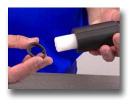
Step 7: Remove the anti-lock ring.
