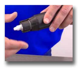
**Step 20:** Reinstall the check valve nut. Set the stem aside.
