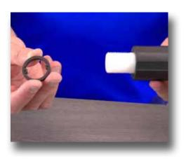
**Step 17:** Then, align the teeth inside the anti-lock ring with the grooves on the white stem and slide it onto the bottom of the stem.
