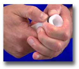
**Step 10:** Now, remove the injection Stem o-ring (Part #: JDI098) by pinching and rolling it off of the white stem. Install the new o-ring into the groove.
