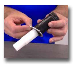
Step 14: Slide the metal retainer onto the sleeve.
