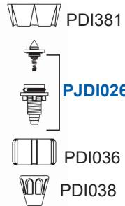
2. Unscrew the suction hose nut (PDI038) and check valve nut (PDI036). Pull out the check valve assembly (PJDI026) noting orientation of inner check valve cone with spring.
